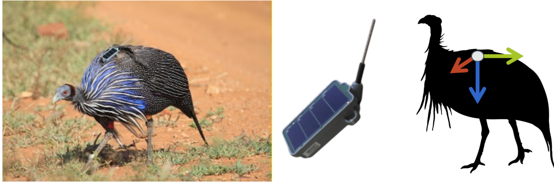
Figure 7: A tagged vulturine guineafowl with the e-obs device. The acceleration is measured along the three illustrated axes
