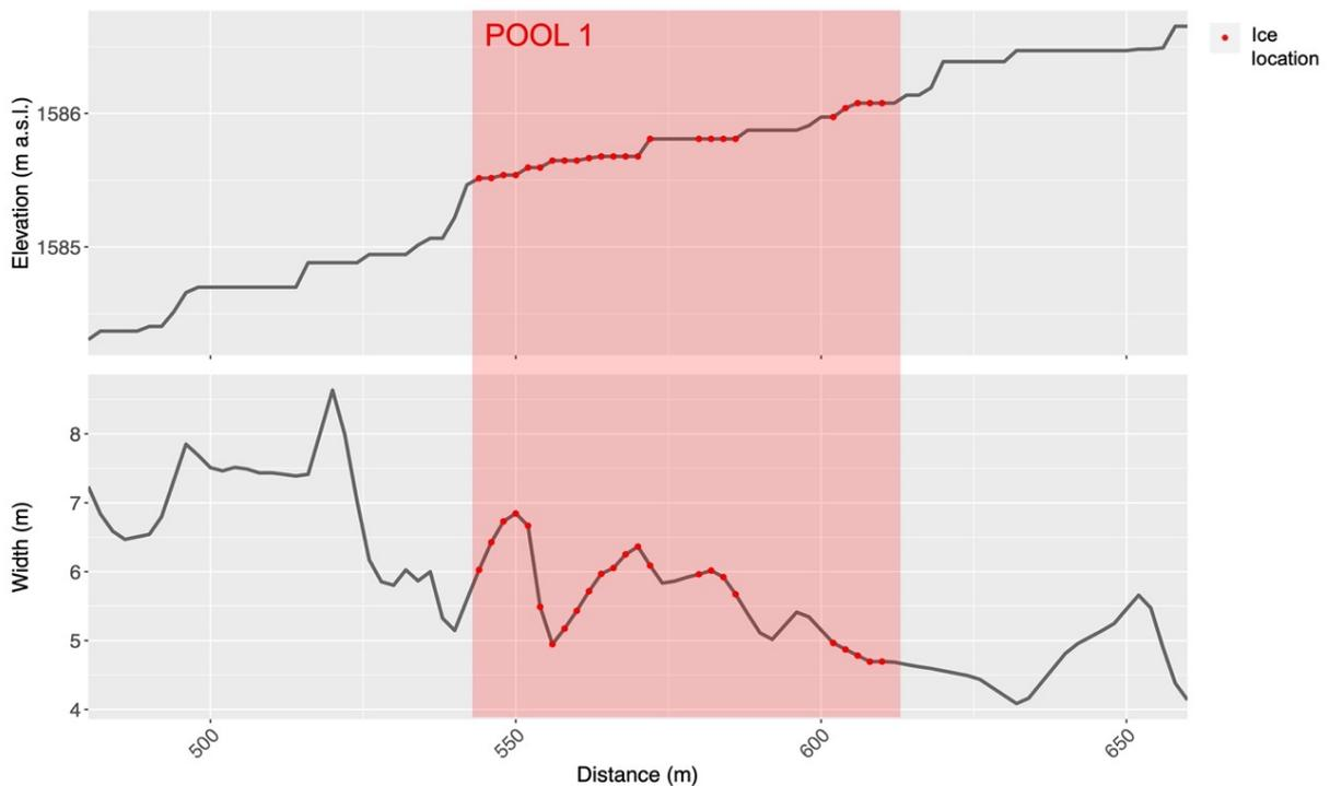
Figure 5.2: Stream elevation and stream width along the Dischmàbach every 2 m around the location of Pool 1 (red area) and the locations showing a rise in the water level (red dots)
