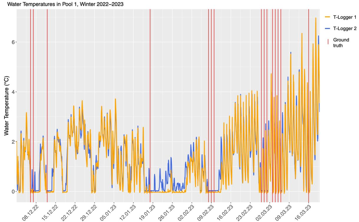
Figure 5.6: Water Temperature in Pool 1 between December 2022 and March 2023, one near the morphological step (T-Logger 1) and the second further behind the morphological step (T-Logger 2)
