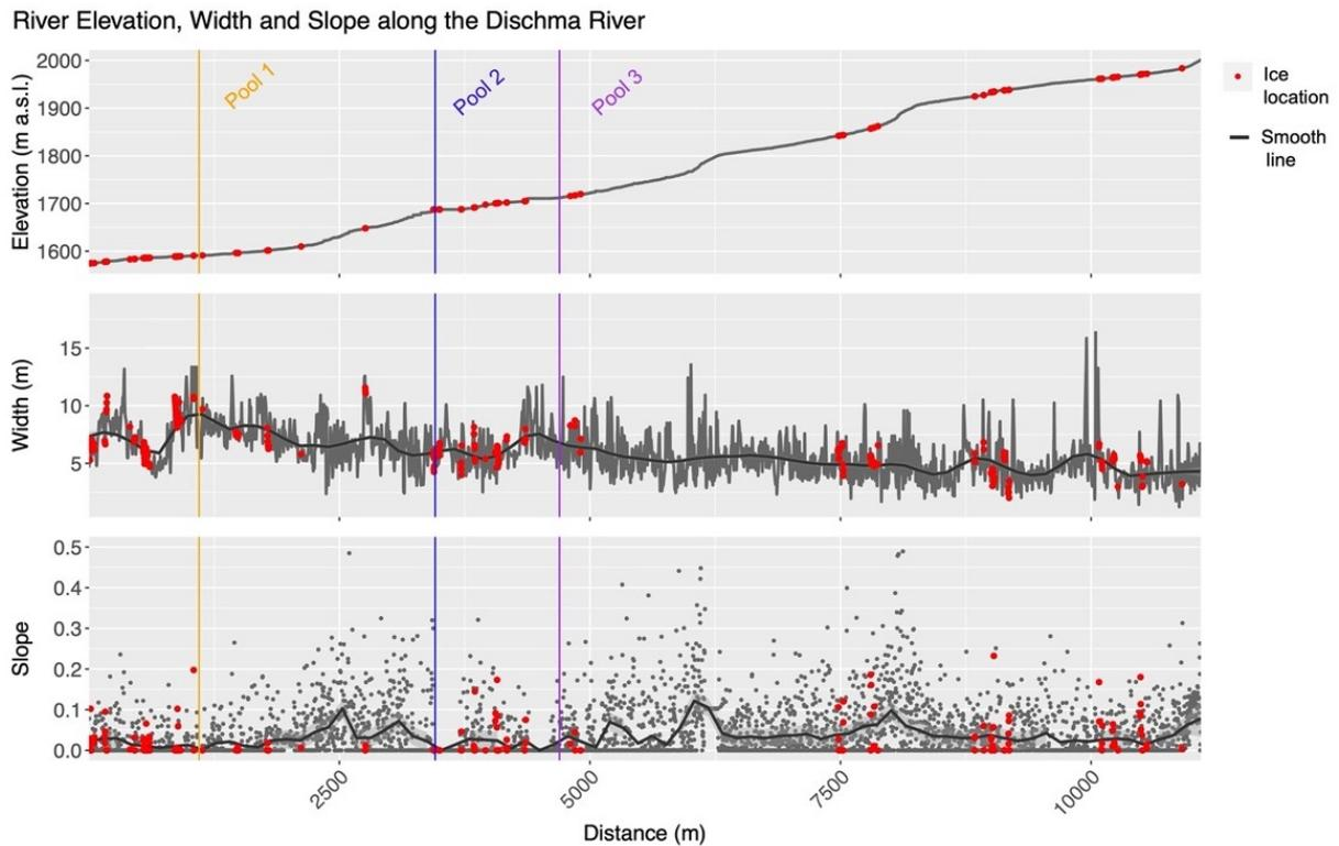
Figure 5.1: Elevation, width, and slope along the Dischmàbach measured/calculated for every 2 m and the locations showing a rise in the water level (red dots)
