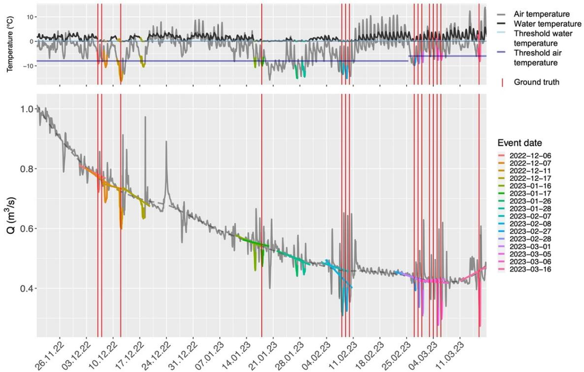
Figure 5.14: Overview of the found events by the algorithm with the *exponential decay* No-Ice-Model and a pre-time of 5 days with the events detected by the wildlife camera (red lines)
