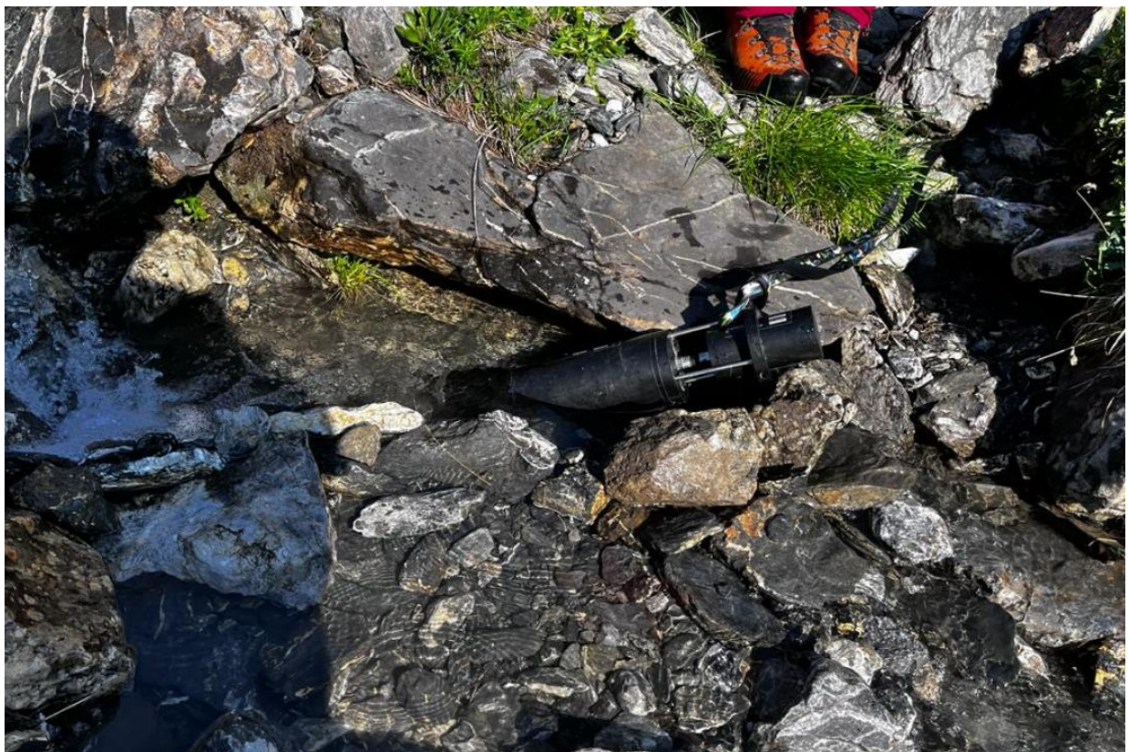
Appendix 6: Fluorometer placed at KL-WHQ during KL-23-01-CBP-Ur.
