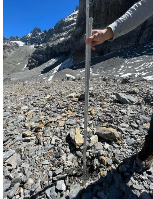
Figure 17: Measurement of an ablation stake on Griess Glacier using a twin meter.
