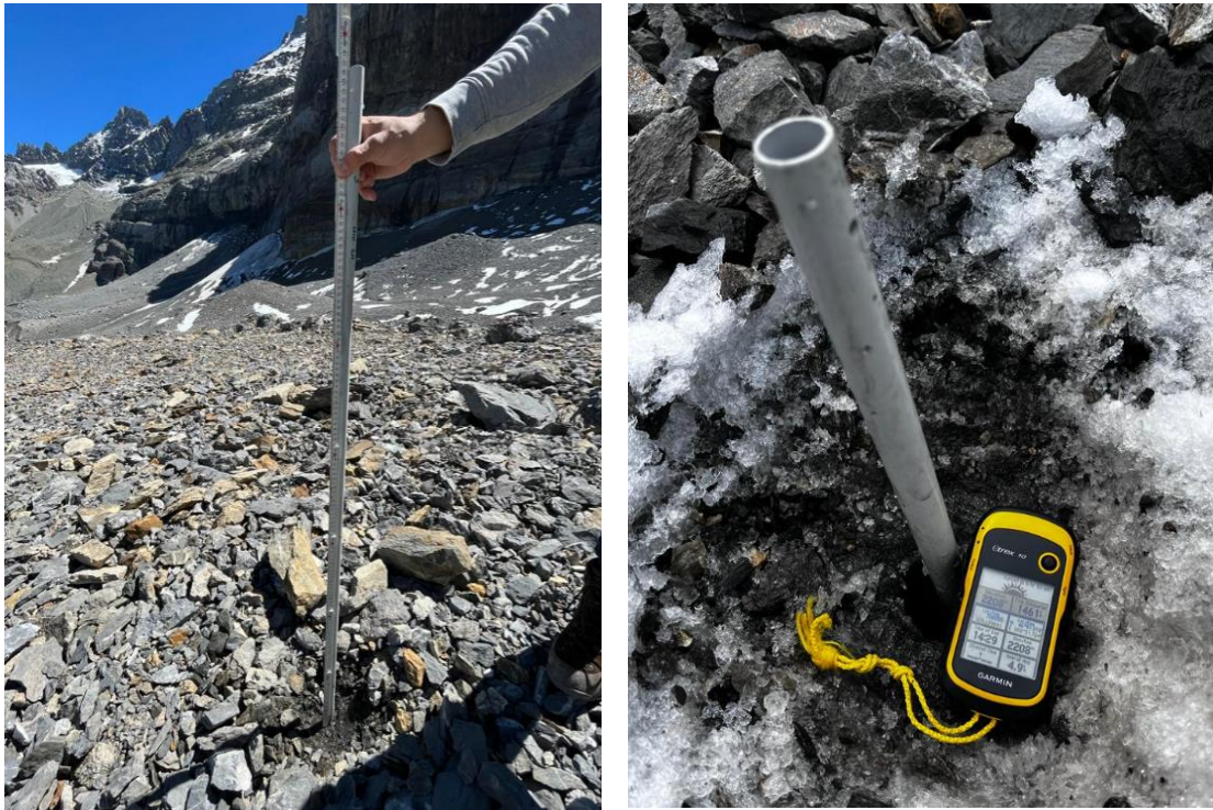
Appendix 11: Ablation stakes drilled into the ice of Griess Glacier.
