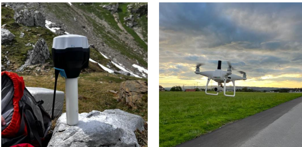
Figure 16: Left: The Emlid basestation set up on the moraine bastion north of the Griesseeli. Right: The DJI Phantom 4 Pro V2 in mid-flight. The black cylinder on top is its build-on PPK antenna.
