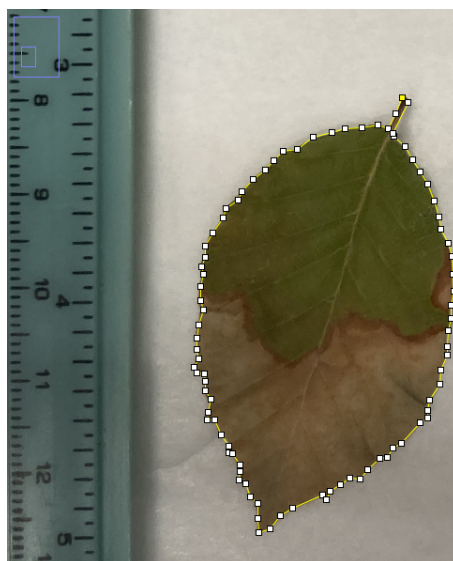
Figure A.6: Leaf area estimation in ImageJ using the point tool and a known distance scale.
