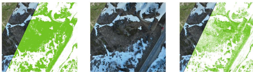
Figure 35 (a), (b) and (c): Snow cover map created using Red derived NDVI, aerial view and Red-Edge derived snow cover map.
