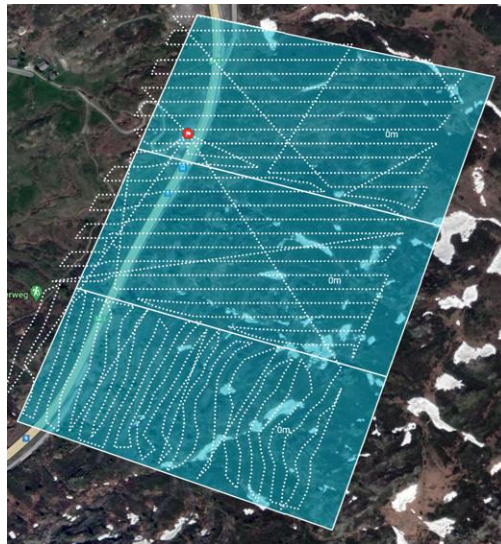
Figure 13: Flight plan visualized in the Drone Harmony interface. Each blue rectangle corresponds to a single flight while the white lines trace the path followed by the drone.
