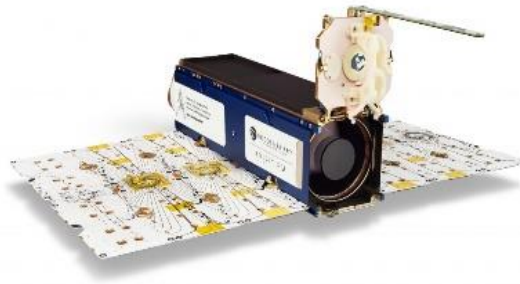
Figure 9: One of the SuperDove satellites part of the PlanetScope Constellation. Image credit: Planet Labs.
