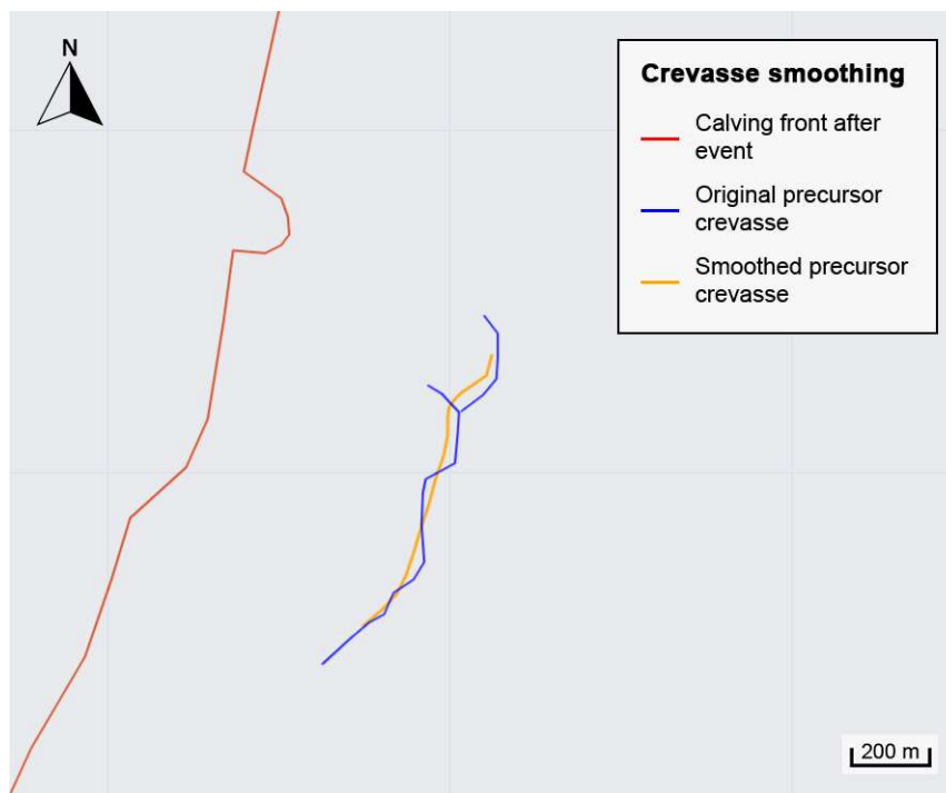
Fig. 17: A smoothing algorithm is applied to calculate an average line (in orange) representing the precursor crevasse (blue line). The result allows for a better distance calculation to the calving front (red line).
