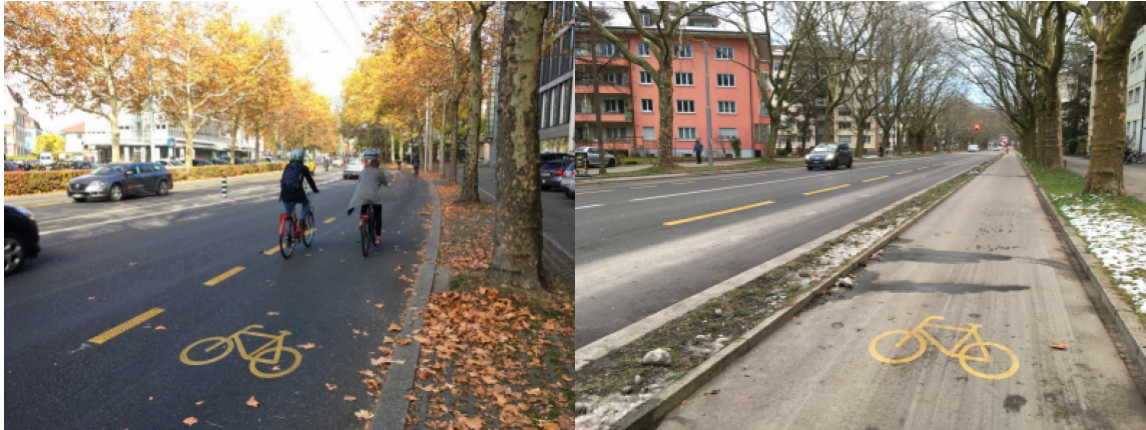
Figure 5 Cycle lane (left) and cycle track (right). Illustrations by Rérat et al. (2023).
