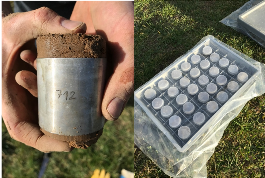
Figure 6: Left: Filled soil core sample ring. Right: Storage box for transportation filled with several soil core samples. Source: Own photos.
