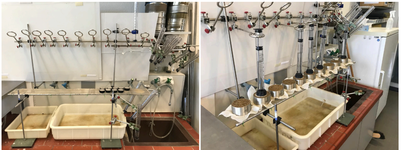
Figure 8: Left: The empty apparatus for the hydraulic conductivity measurements with space for 10 Mini tension disk infiltrometers. Right: Apparatus with 10 soil core samples in place. Source: Own photos.
