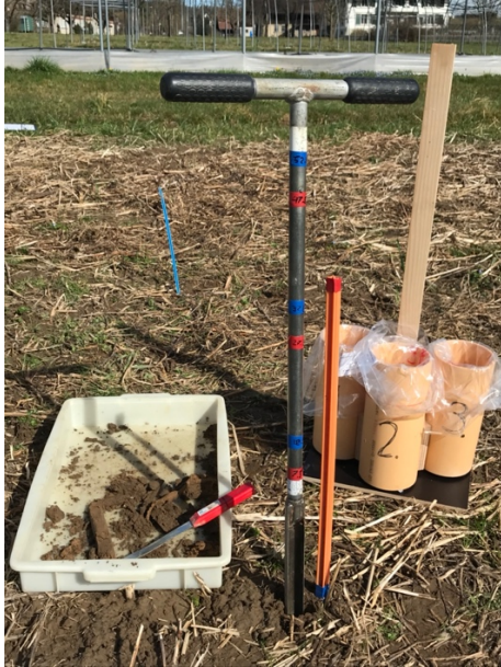
Figure 7: Setup for measuring the composite samples in the field. Source: Own photo.
