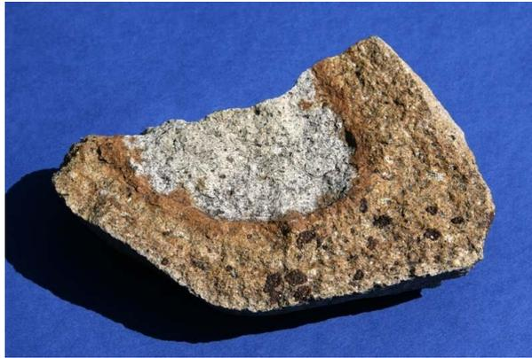
Fig. 8: Weathering rind of a granite (source: <http://geologypics.com/we-29/>, 22.08.2018).
