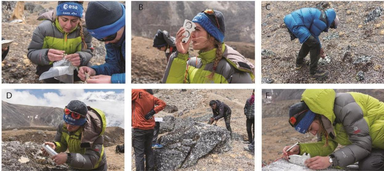
*Fig. 18: Field measurements; A: weathering rind; B: topographic shielding; C+D: Schmidt-hammer; E: cutting rocks out with hammer and chisel; F: strike and dip; Photos: Pierre Lecomte, ESA photographer.*
