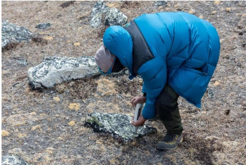
Fig. 10: Conducting rock hardness measurements with the Schmidt-Hammer (Photo: Pierre Lecomte, ESA photographer).
