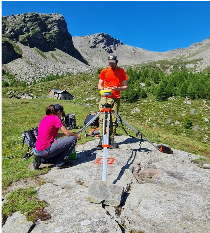
Figure 10: Installation of the base station on a stable terrain outside the rock glacier. Photo: S. Crivelli. Date: 26.06.2023.
