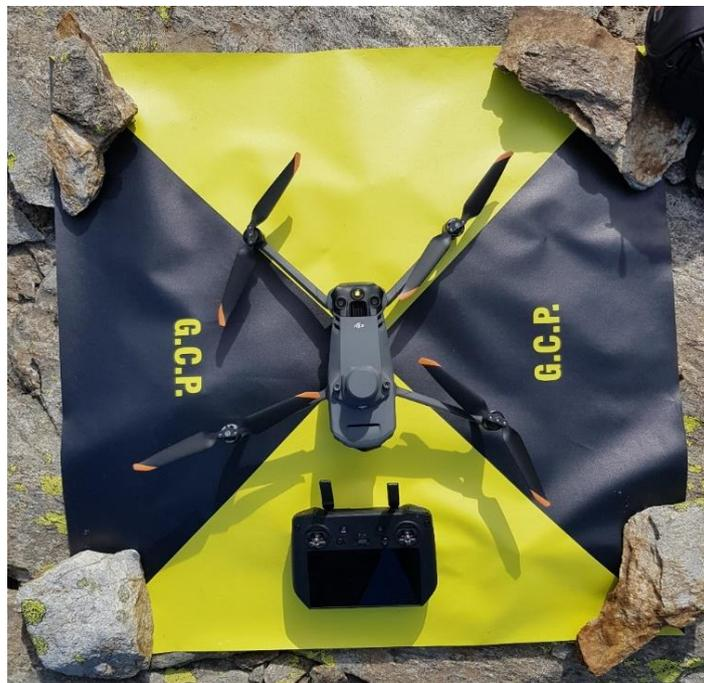
Figure 14: Ground Control Point, drone, and controller.
