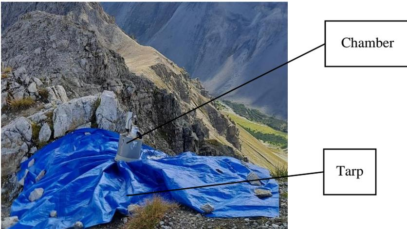
Figure 10: Soil respiration measurement cylinder on grass (upper picture) and cylinder with tarp on bare rocks (lower picture)
