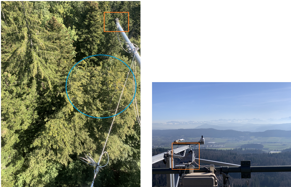
Figure A.1: The FloX setup in the Lägeren measurement station. The left picture shows the FloX FOV on three beech trees from the tower in the blue circle and the downwelling radiance sensor in the orange square. The right figure depicts the on tower setting with the FloX box and the upwelling radiance sensor in the orange square. Source pictures: Michael Niederberger (Remote Sensing of Water Systems, Department of Geography, University of Zurich, 2024).
