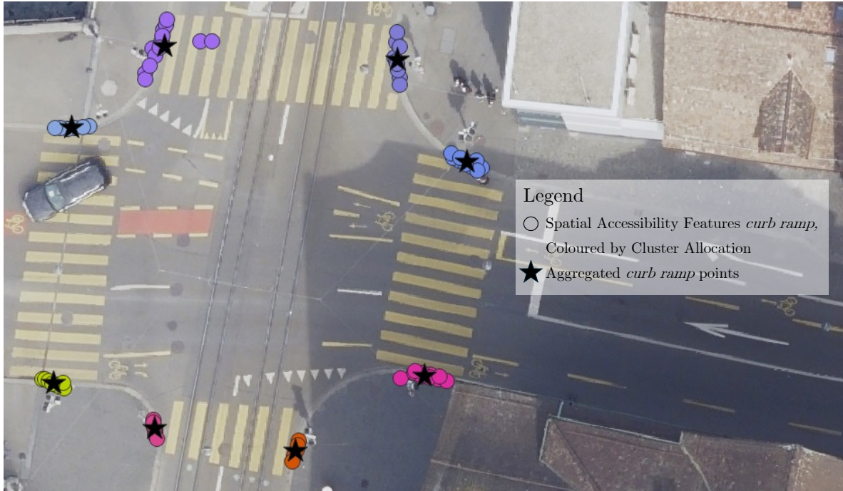
Figure 4.4: Resulting spatial accessibility features curb ramp clusters, created by hierarchical clustering, and aggregated curb ramp points (Areal image: Kanton Zürich (2020))
