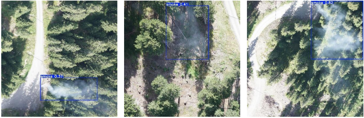
Figure 4.2: Examples of false positives smaller area (above) compared to true positives bigger area (below)
