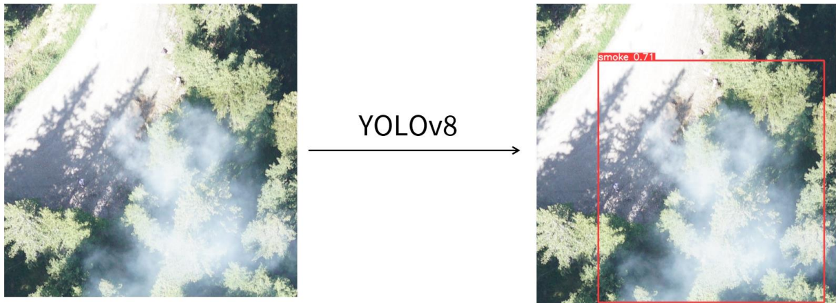
Figure 2.7: Example of a 1000x1000 pixels segment (left) and the detection result (right) after being processed through the YOLOv8 pretrained model
