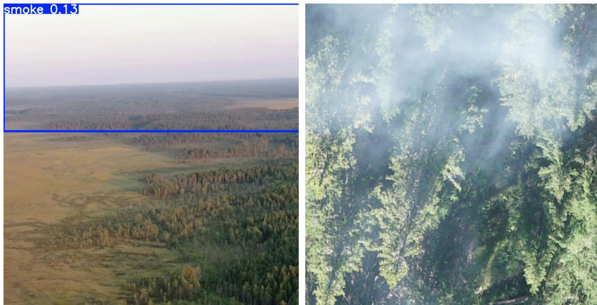
Figure 4.3: A false positive detected in the “Flame 2” dataset (Hopkins et al., 2023) by the tuned algorithm caused by the grey sky opposed to the green vegetation (left) and a segment of image used for the third phase of the tuning process that sees grey smoke opposed to green vegetation (right)
