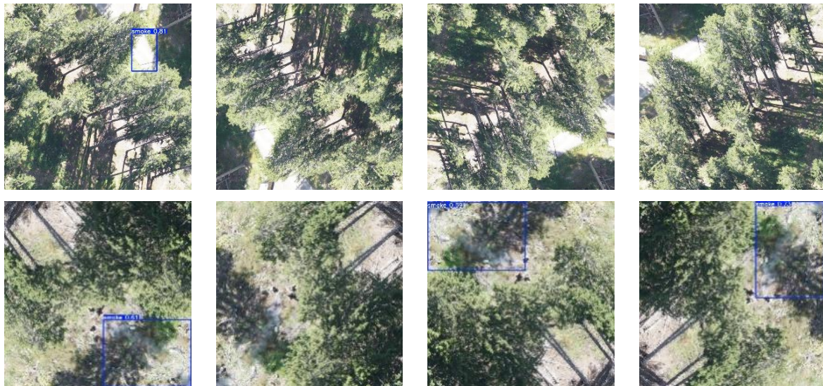
Figure 4.1: Example of a false positive showing detection only in one of the four rotations (above) and a true positive showing detection in three out of four (below)
