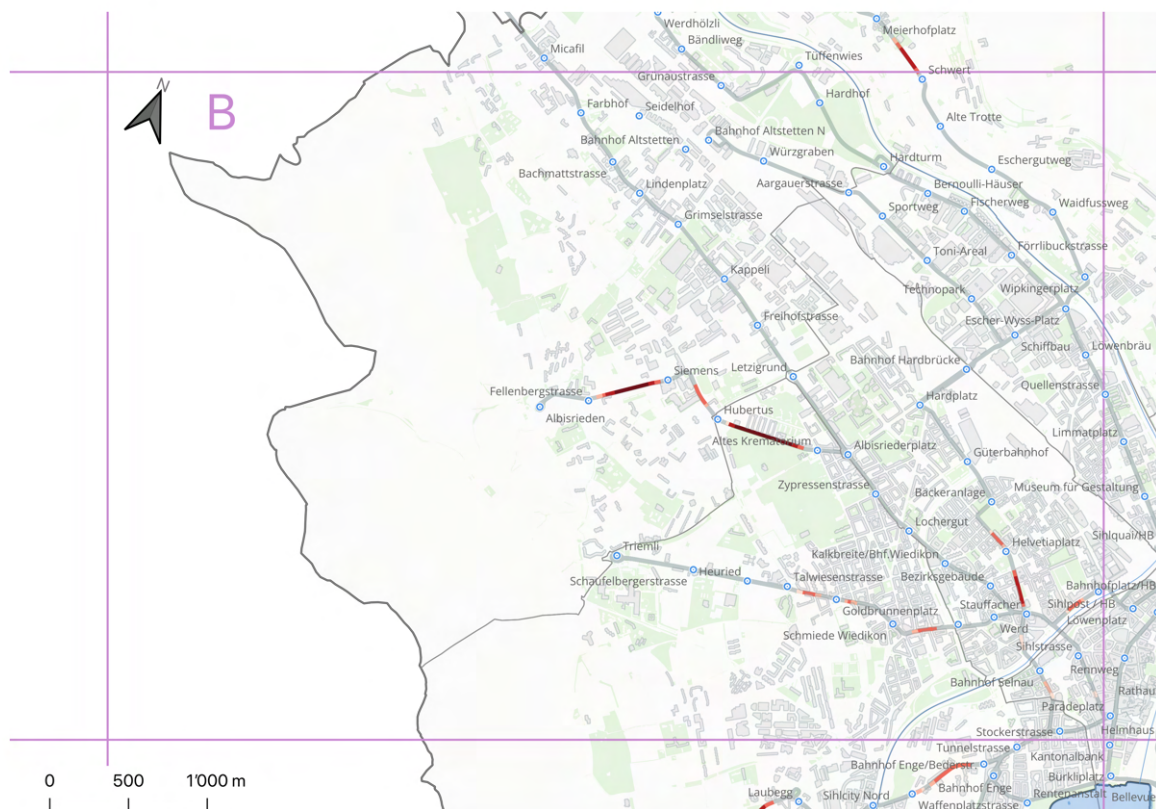
Figure C.5: Additional time need (in s) for trams in Grid B during HVZ1, Direction 2, in 20-meter segments. See Figure C.17 for detailed legend.
