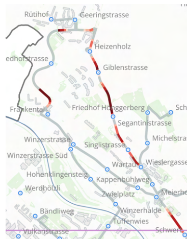
Figure 5.3: Detailed view of additional time need between stops Schwert and Frankental for bus in HVZ1 Direction 1
