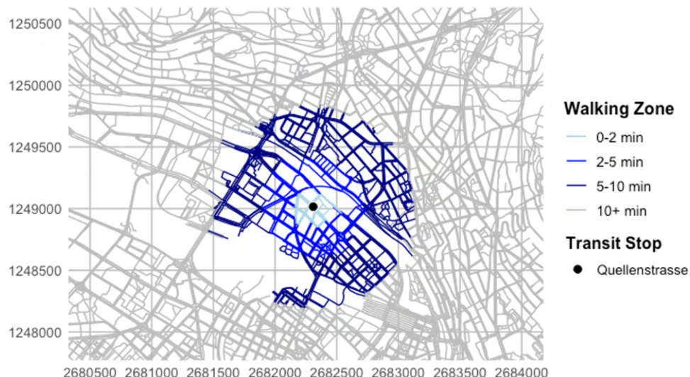
Figure 5.28: Walking zones from stop Quellenstrasse , categorized into walking time classes of 0–2 min, 2–5 min, 5–10 min, and +10 min.
