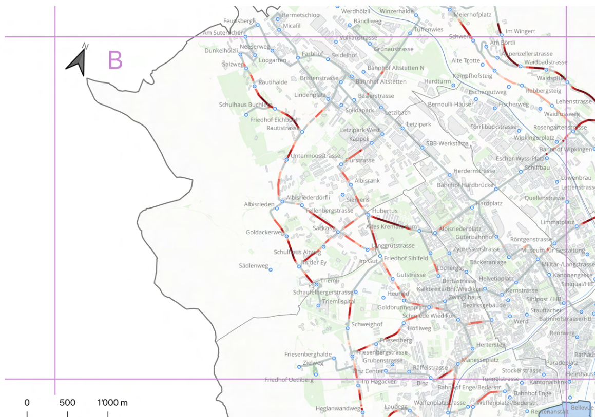
Figure 5.6: Additional time need (in s) for buses in Grid B during HVZ1, Direction 1, in 20-meter segments. See Figure 5.16 for detailed legend.
