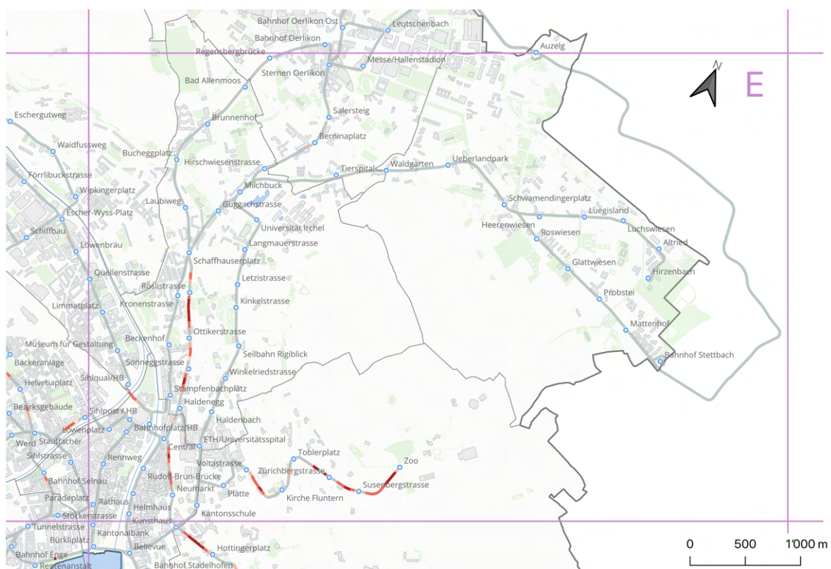
Figure C.14: Additional time need (in s) for trams in Grid E during HVZ2, Direction 2, in 20-meter segments. See Figure C.18 for detailed legend.
