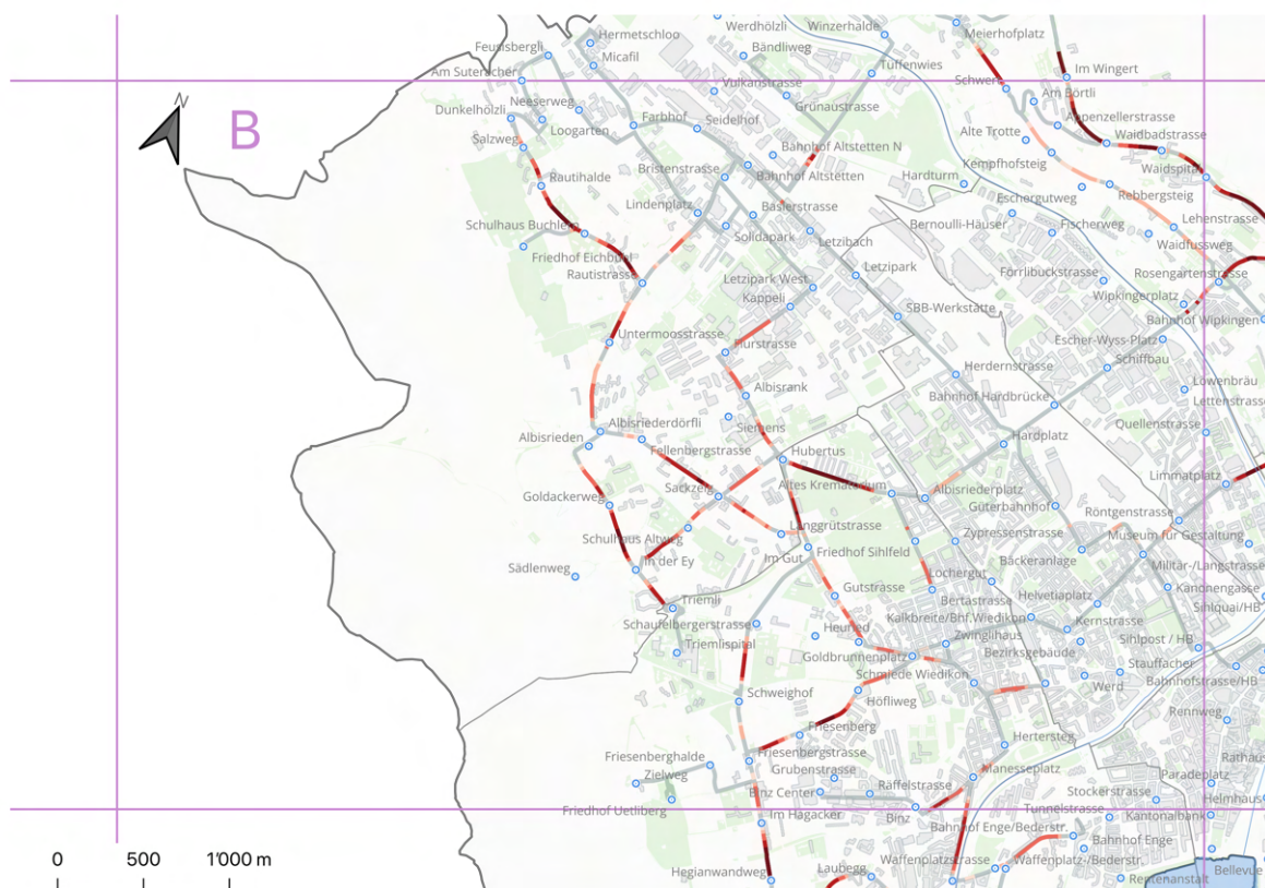
Figure 5.7: Additional time need (in s) for buses in Grid B during HVZ2, Direction 1, in 20-meter segments. See Figure 5.17 for detailed legend.
