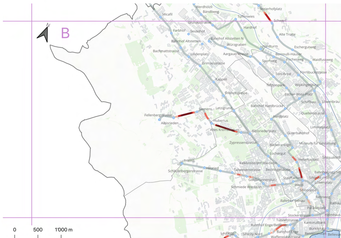
Figure B.5: Additional time need (in s) for trams in Grid B during HVZ1, Direction 1, in 20-meter segments. See Figure B.15 for detailed legend.
