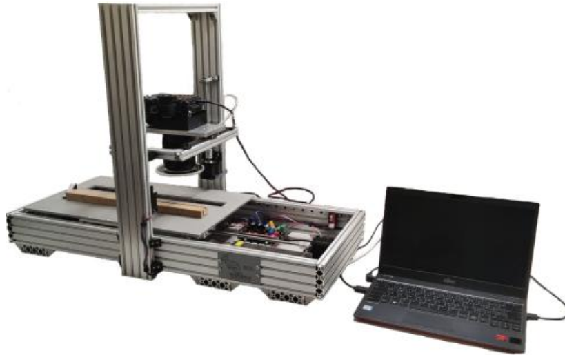
Fig. 20: High-resolution image-capturing system Skippy (source: Gärtner et al., 2024)
