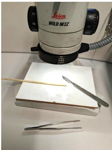
Fig. 24: Cutting the cores (own photo)
