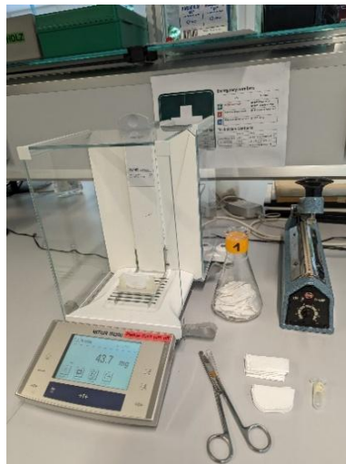
Fig. 25: Weighing into Teflon bags (own photo)
