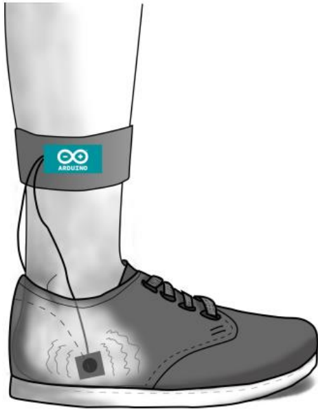
Figure 4: Overview of the Shoe me the Way components: Two vibration actuators are placed near the user's ankle, one on either side of the foot. The actuators are controlled by a microcontroller that is worn at the lower leg (Schirmer et al., 2015).
