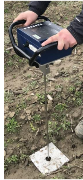
Figure 6: Measurement with the Penetrologger in the field (picture by T. Cigler).
