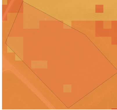
Figure 4.2: Field parcel with underlying grassland use-intensity map at a 10 m pixel resolution. Each pixel indicates the timing and number of management events that have been detected within one year.
