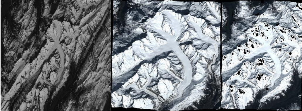
Image 3: Display of single stereo images that were used to produce the Spring Series DEMs . (A) SPOT5 HRS image from 26.03.2003, (B) Pléiades HiRI image from 31.03.2021, (C) Pléiades Image from 11.04.2024.
