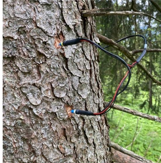
Figure 4. Installation of sap flow sensors into the tree
