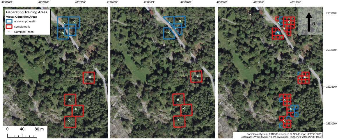
Figure 4.2: Overview of the step-wise approach for generating training areas. The first approach involved creating 30x30 m areas surrounding the sampled trees (left), followed by the second approach which aimed to exclude street segments and non-vegetated land cover (middle). The final approach subdivided the areas into smaller 10x10 m sections (right).
