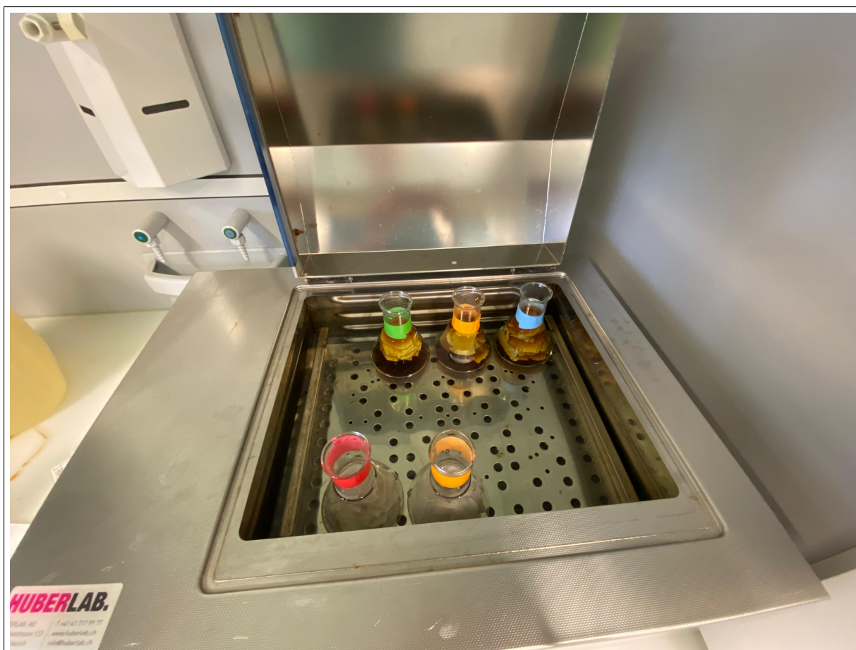
Figure 2.10 Teflon bags in the Erlenmeyer flask in the 60°Celsius water bath (source: own picture).
