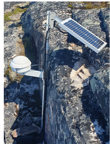
Figure 8: Picture of the time-lapse camera named hill, near the main camp.
