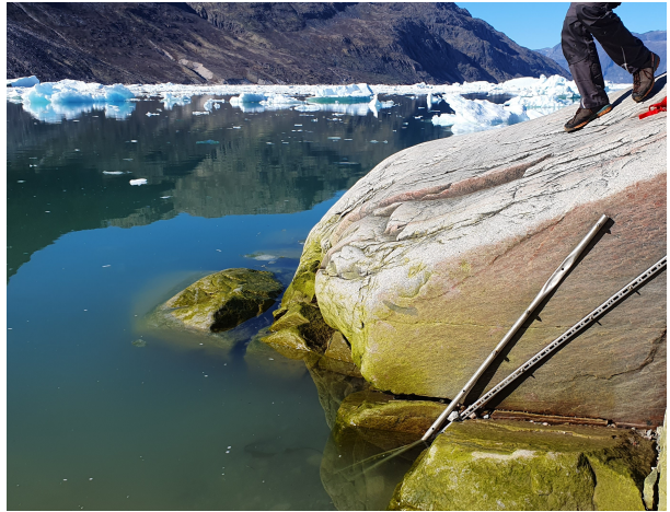
Figure 6: Picture of the tide gauge number 1 (P1), placed into a metal tube and screwed to a rock.
