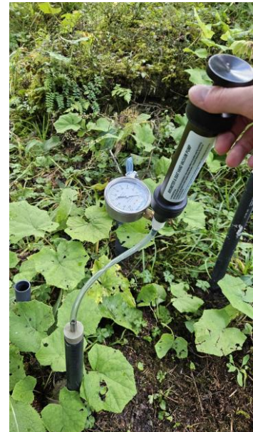
Figure 12: Application of a negative pressure using a hand pump.
