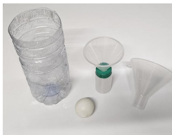
Figure 16: Components of the rainwater collector. The sample was taken from the smaller inner bottle with the green lid.
