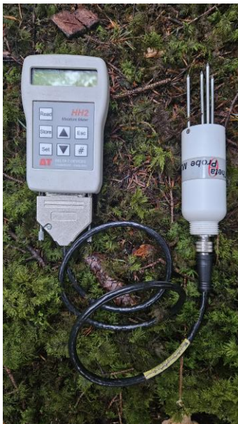
Moisture Meter type HH2 with a ThetaProbe ML3 sensor.
