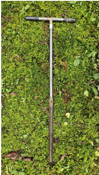
Figure 10: Auger used for lysimeter installation and soil sampling.
