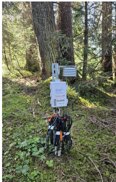
Soil moisture, relative humidity, and air temperature logger at L1.
