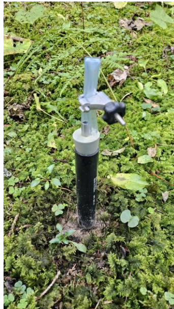
Figure 11: Lysimeter closed with a clamp and sealed with clay.
