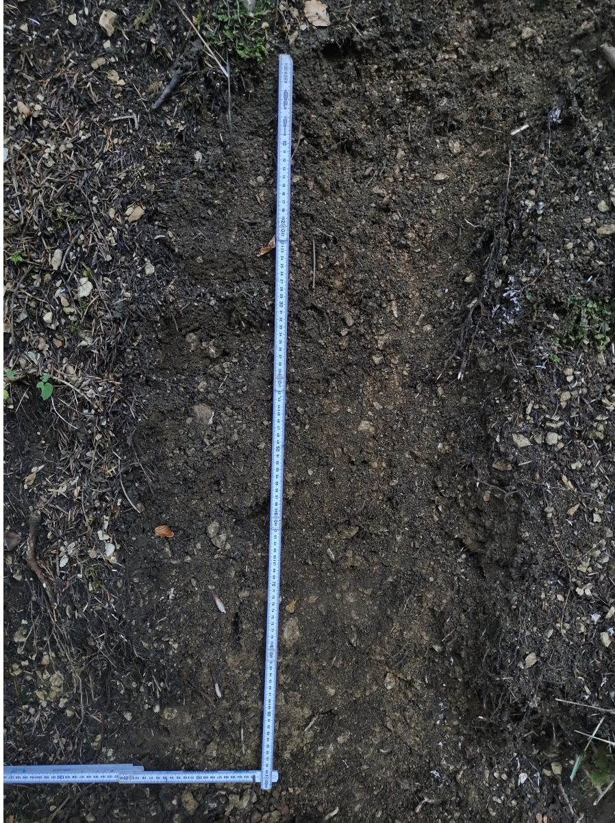
Figure 5: The soil density can be determined by assessing the resistance to penetration in different soil horizons in the profile using a knife. The soil profile was dug at plot 2035000 as the third measurement (own photograph).
