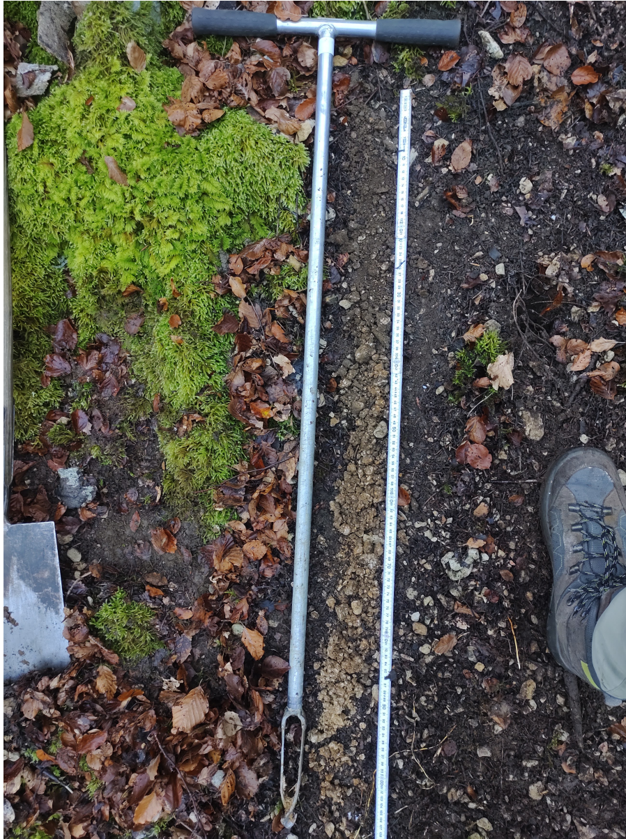
Figure 4: The drill core was evenly laid out on the forest floor, using the folding rule and a handle of the spade or the auger as straight boundaries. This drill core was carried out at plot 2035000 in Buttes (first measurement, own photograph).
