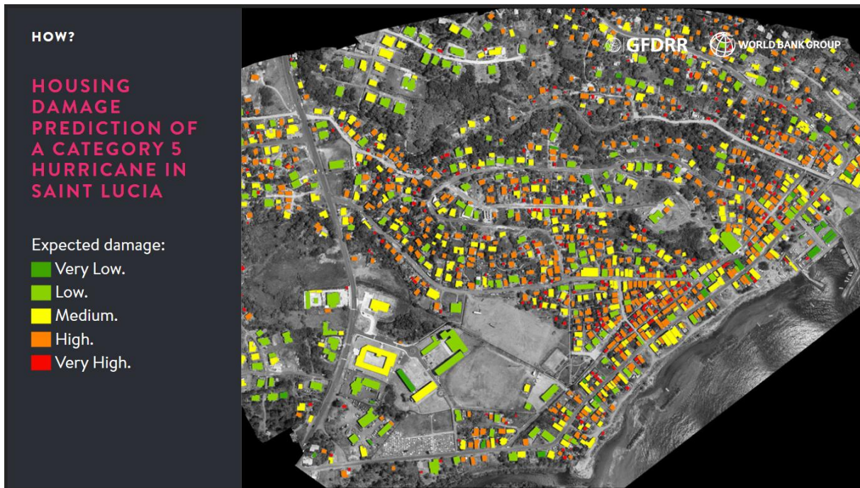
Figure 10: Hurricane Damage Prediction in St. Lucia by the GPRH (Wahba 2018, 28).
