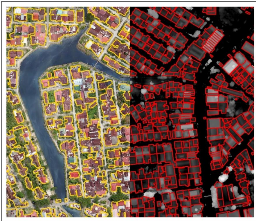
Figure 4. The urban rooftop vector layer, shown in yellow, overlaid on the orthophoto mosaic (left). Clustered rooftops were reviewed and manually divided, if necessary, as shown in red, on top of the digital object model (right) to create a building footprint layer.
