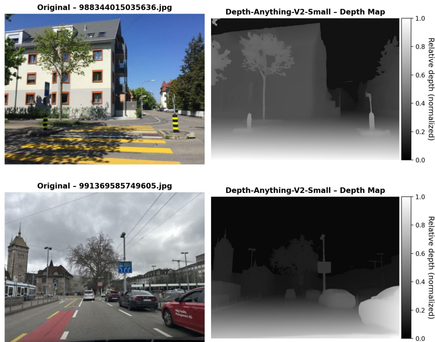
Figure 5.11: Examples of depth estimation outputs on different scenes: original images (left) and corresponding depth maps (right).
