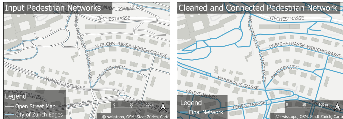
(a) Input pedestrian networks (OSM and City of Zurich). (b) Final merged and cleaned pedestrian network.
