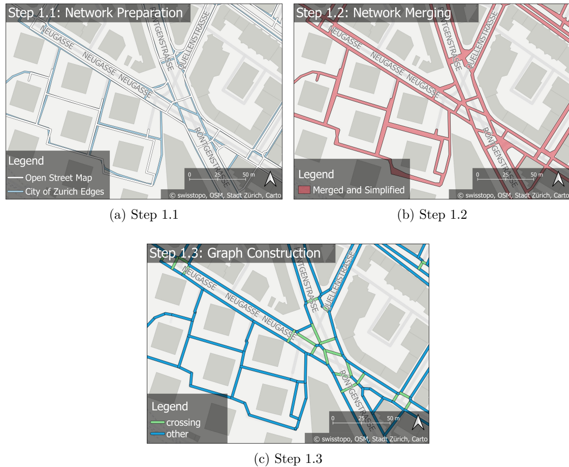
Figure 4.3: Illustration of Phase 1: Network Model Development. Subfigures show (1.1) network preparation using OpenStreetMap and City of Zurich data, (1.2) merging and simplification of overlapping network segments and (1.3) graph construction with classification of sidewalks and crossings.
