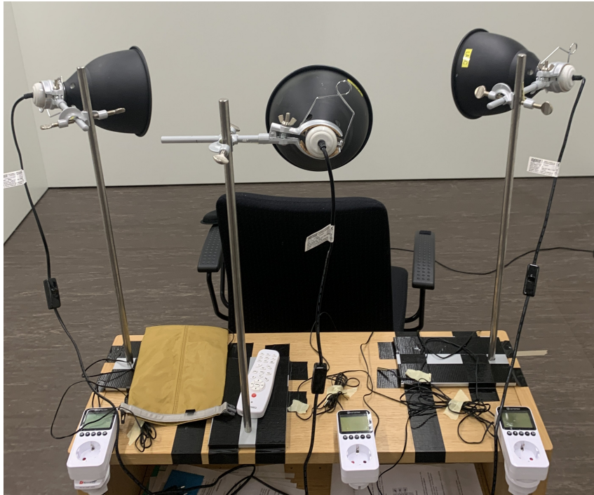
Figure 3.4: Thermal manipulation apparatus components and mounting geometry, including Philips infrared lamps, thermostats, and safety sensors.
