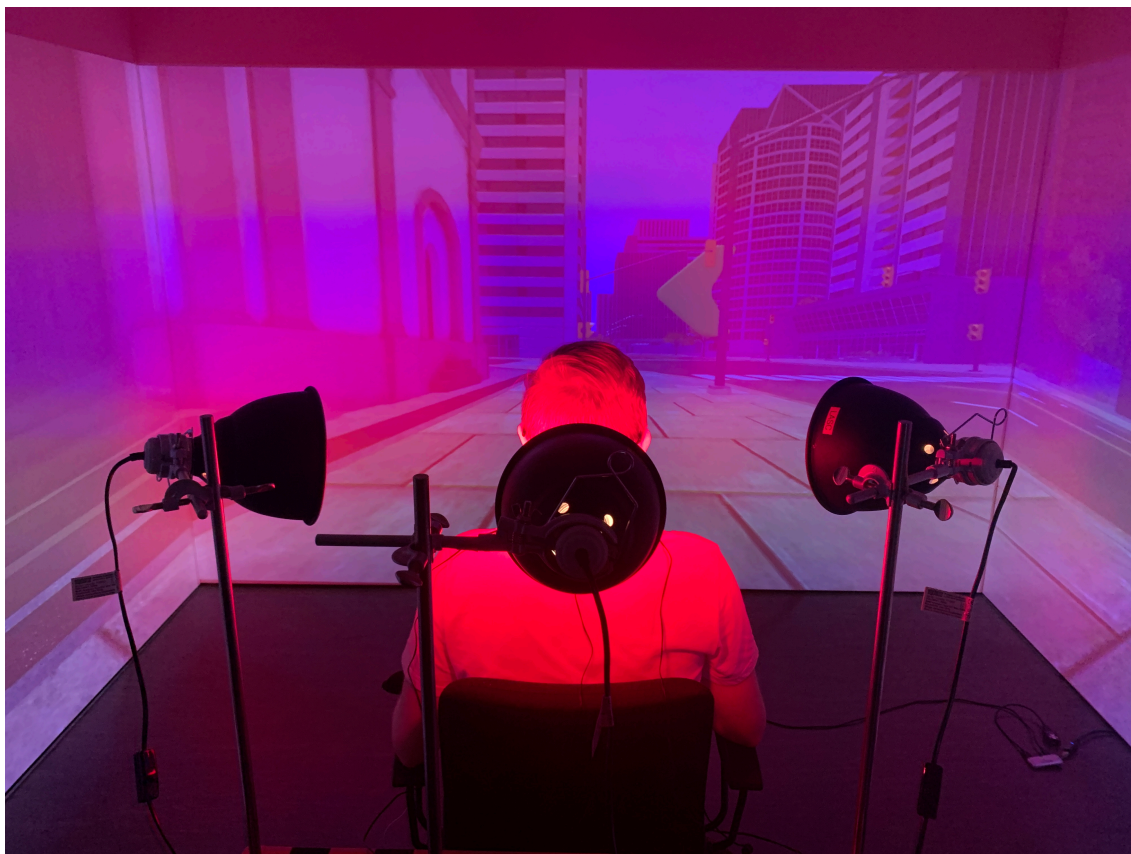
Figure 3.3: Experimental setup in the CAVE displaying the thermal apparatus: three Philips infrared lamps (left, right, posterior) positioned around the participant's head and neck, controlled by independent thermostats to maintain target heat exposure (36-38°C). The virtual urban environment is projected on the surrounding screens.
