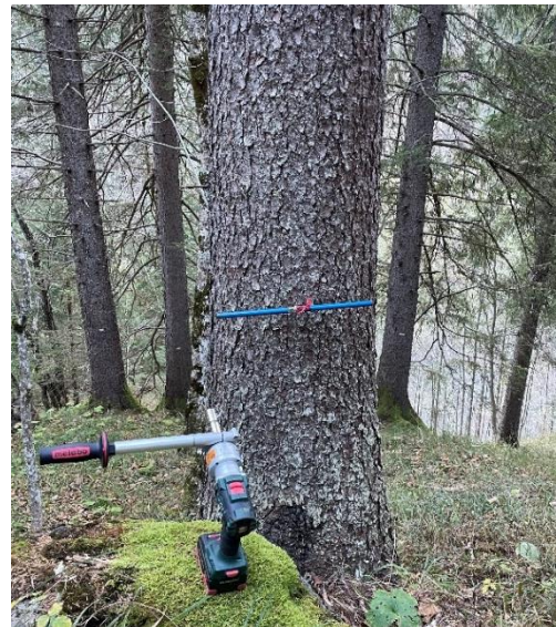
Figure 16: Photograph of sample Elm105 and sampling equipment (Pressler Bohrer, extractor, and power drill).
