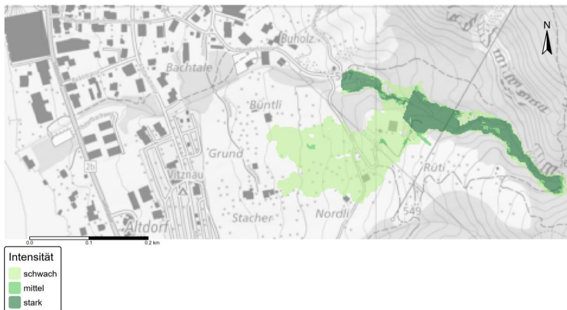
Figure 35 Intensity map of the Altdorfbach and Vitznau for the 100-year scenario including climate change adjustment after construction of the new dam and connection to the old structure.
