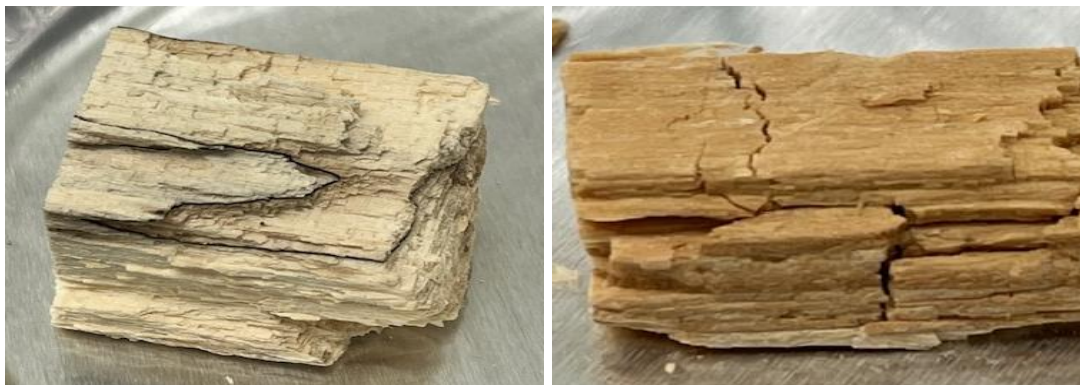
Figure 4: White rot decay of hardwood and brown rot decay of softwood (from left to right). Note. Created by the author.
