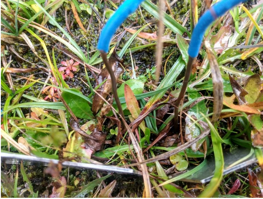
Figure 3 ER sensor with its two electrodes including the V-shaped metal plates.
