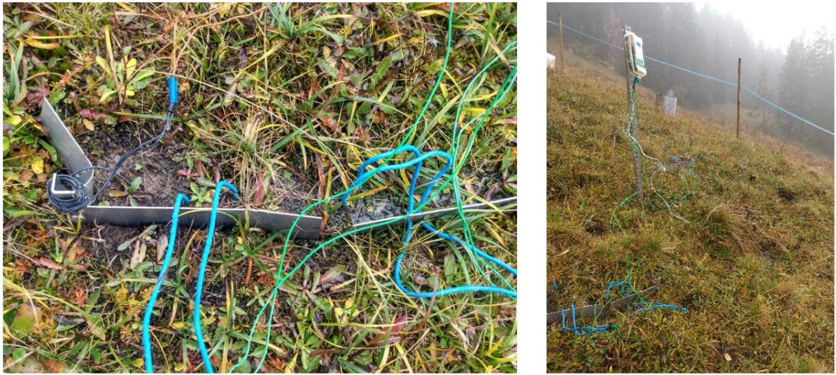
Figure 4 Field setup with metal plate (left) with the V-shaped configuration including the two electrodes placed in the 5 cm gap. Microcontroller board (right) with the OF1 and OF2 installed on each side.
