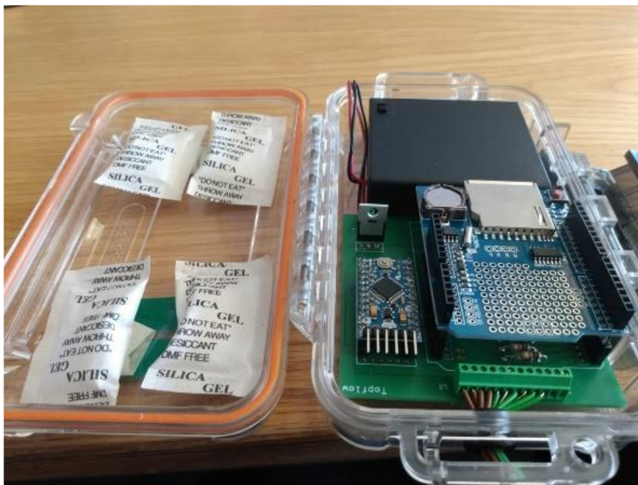
Figure 2 Microcontroller board and SD card data logger shield.
