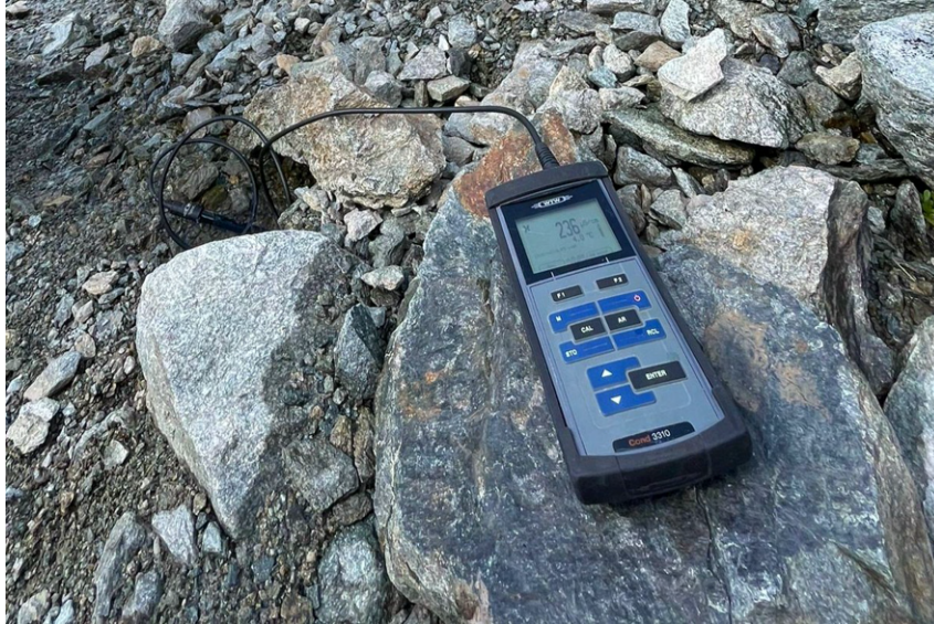
Figure 18: Handheld measurements with a WTW Cond 3310 (Ilja van Meerveld, 2025).
