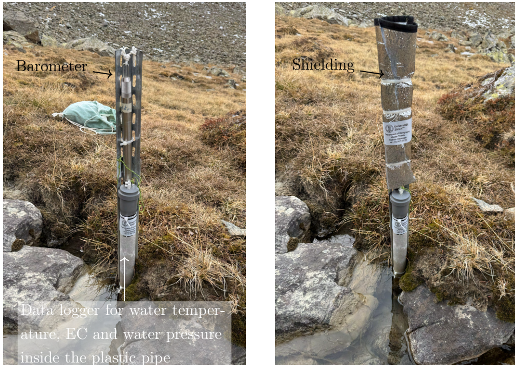
Figure 16: Photos of the automatic monitoring station in front of the Muragl rock glacier with and without the shielding of the barometer (Kathrin Habegger, 2025).
