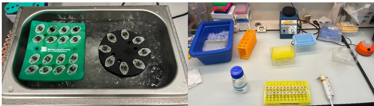
Figure 17: Chlorophyll analysis in pictures. Sonicating water bath with ice (left), and pipetting into 96-well plate setup (right). Picture by Cedric Gehrler.
