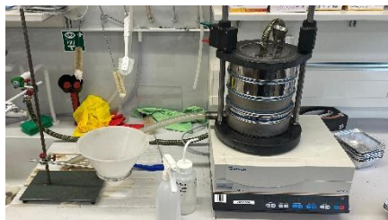
Figure 9: Wet aggregate stability testing setup. With nesting sieves inserted. Picture by Cedric Gehrler.
