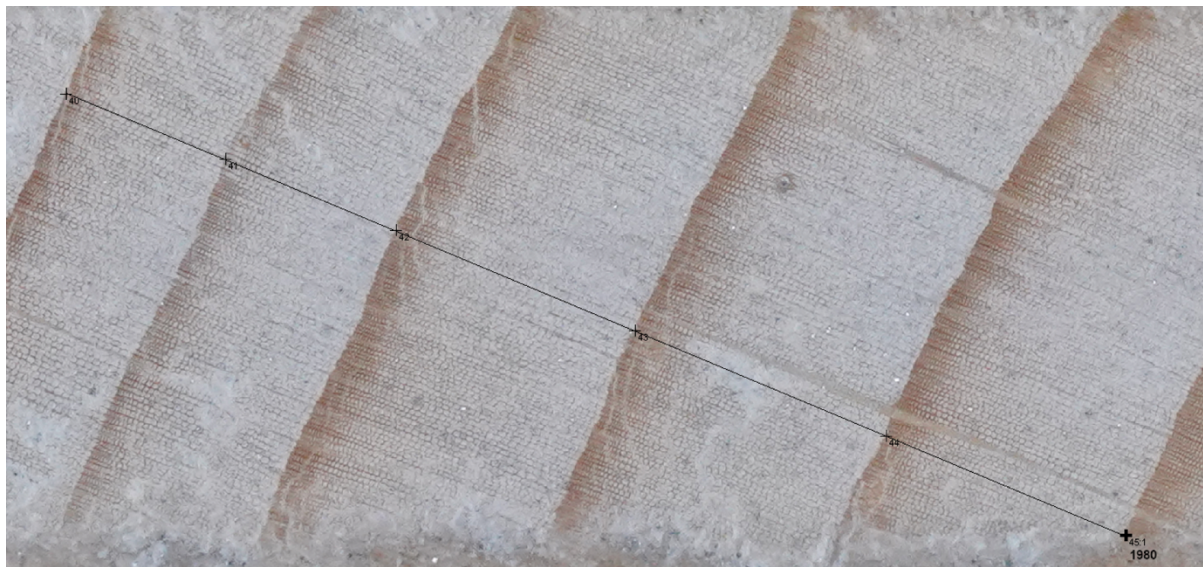
Figure 11: Image of an increment core in Coorecorder with coordinates at ring boundaries.
