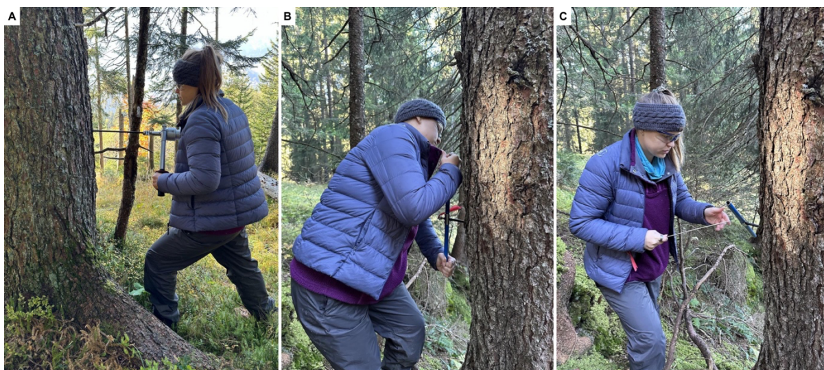
Figure 7: Images from the coring process. (A) shows the initial drilling perpendicular to the tree stem. (B) shows manual turning of the corer. (C) shows the retrieval of the increment core.
