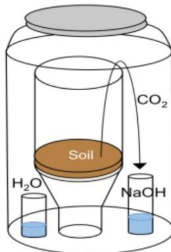
Figure 7: Experimental set up of incubations experiment. Each jar contained a water vial, a NaOH vial and the soil samples where roots had been picked out (adapted figure from Master's Thesis of Jessica Abt, 2017)
