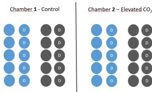
Figure 6: Schematic representation of arrangement of columns in chamber 1 and 2 in MICE. Blue colour represents soil 1 and grey colour soil 2. Columns with a high SBD ( $1.2 \text{ g/cm}^3$ ) are marked with the letter D, all other columns have SBD of  $0.9 \text{ g/cm}^3$
