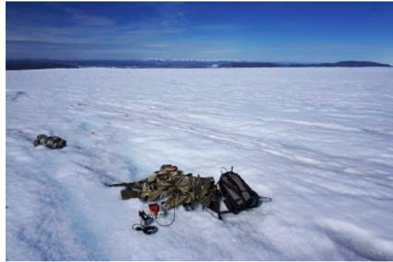
Figure 34: Differential GPS measuring of old EGIG tarps as in-situ control measurements of DEM-derived velocity detection. Note that they are partly frozen to the ice and are therefore not easily moved by wind.
