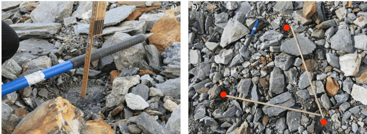
Figure 13. Setup for the debris thickness measurements. a) Horizontally placed pickaxe and folding meter. The debris thickness is measured at the lower level of the pickaxe shaft. b) Three debris thickness measurements (red dots) with a respective distance of 1 m to each other were taken and averaged to compose one single measuring point of debris thickness.
