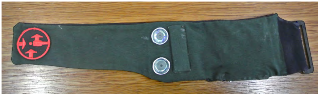
Illustration 5: The inner side of the Smartband with two electrodes.
