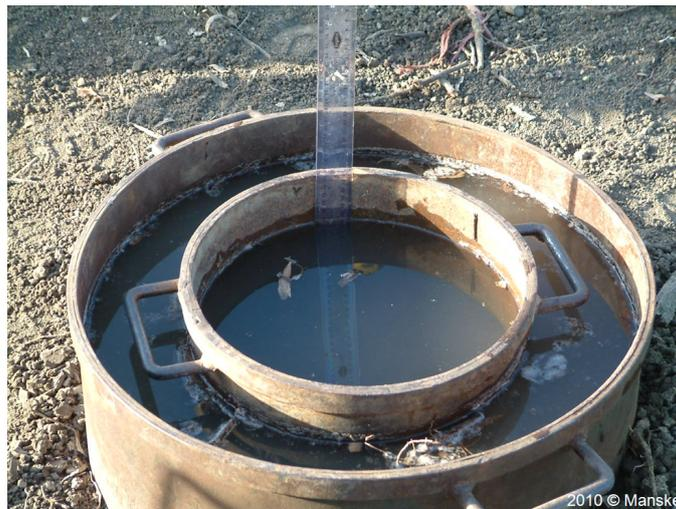
Figure 7: Example of a double-ring infiltrometer construction as used in this study
