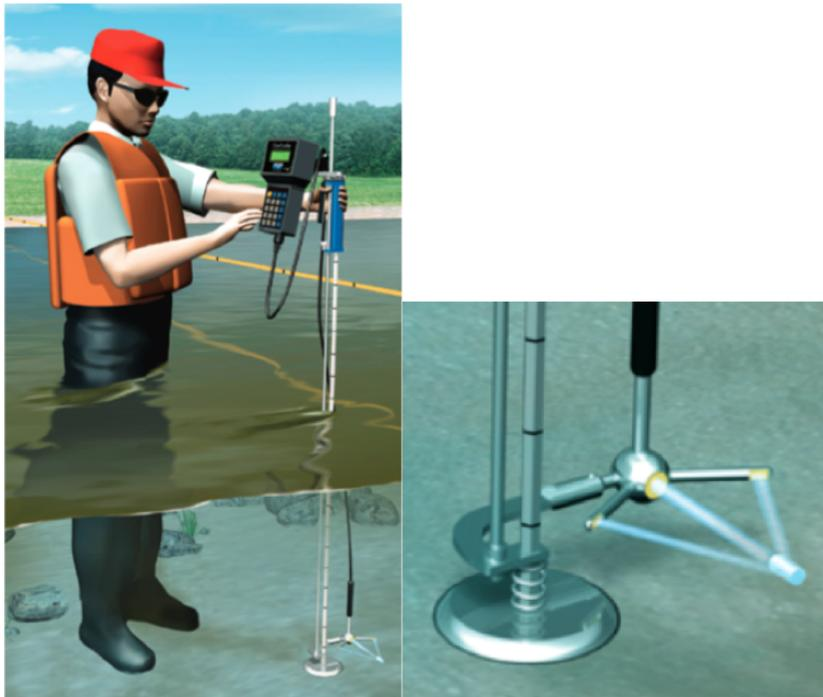
Figure 12: Schematic figure of a Flow Tracker (Quantum Hydrometrie, 2012)
