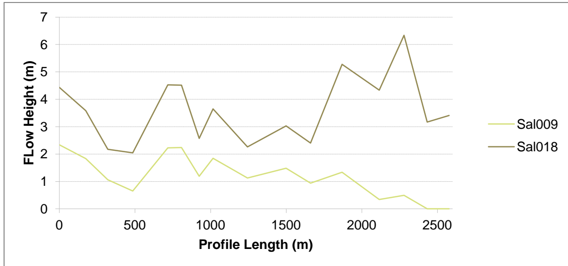
Figure 8.4: Flow heights in the deposition zone near Santa Teresa for different scenarios from Salcantay.
