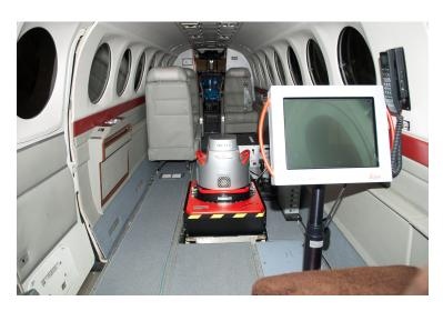
**Figure 3.2:** The ADS80 sensor employed in a Beechcraft Super King Air (©swisstopo).
