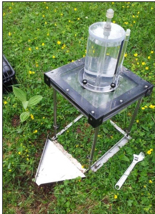
Figure 21 Rainfall simulator installed at the study site Spinas (Source: P. Polich).
