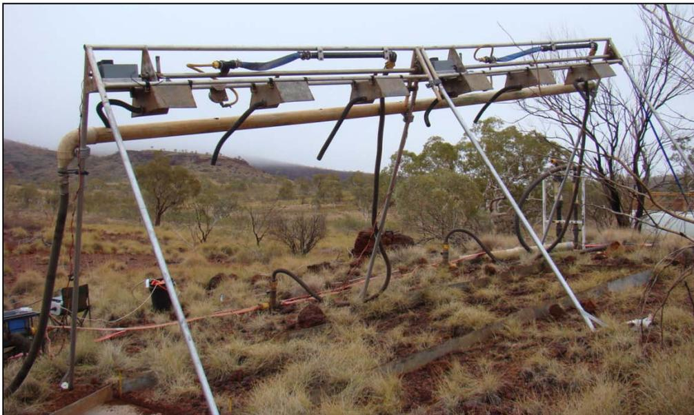
Figure 5 Example of a spray-type rainfall simulator (Source: Landloch).
