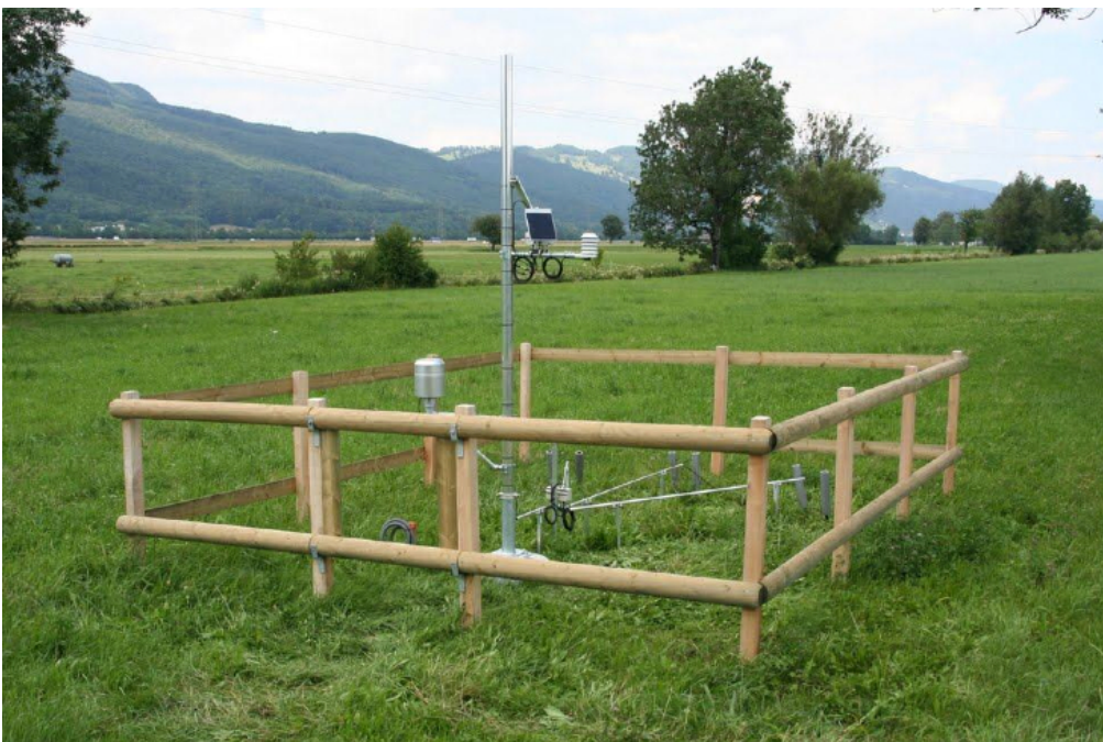
Fig. 4: Soil monitoring network (BMN) station in Kestenholz, SO. The station is operated with solar power only and the data is submitted to the server via GPRS mobile network. Picture: FS BS.
