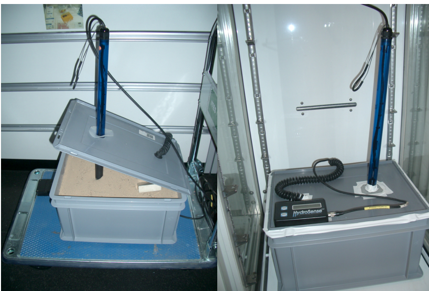
Fig. 34: Plastic box with Winzlerboden soil, T8 and HydroSense open (left) and sealed with plastic tape inside the climate chamber (right).
