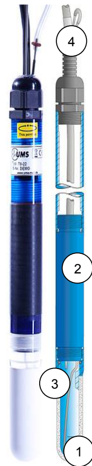
Fig. 13: T8 tensiometer with 1) water-filled cup 2) fibreglass reinforced shaft 3) pressure transducer and 4) refill tubes (UMS, 2008).
