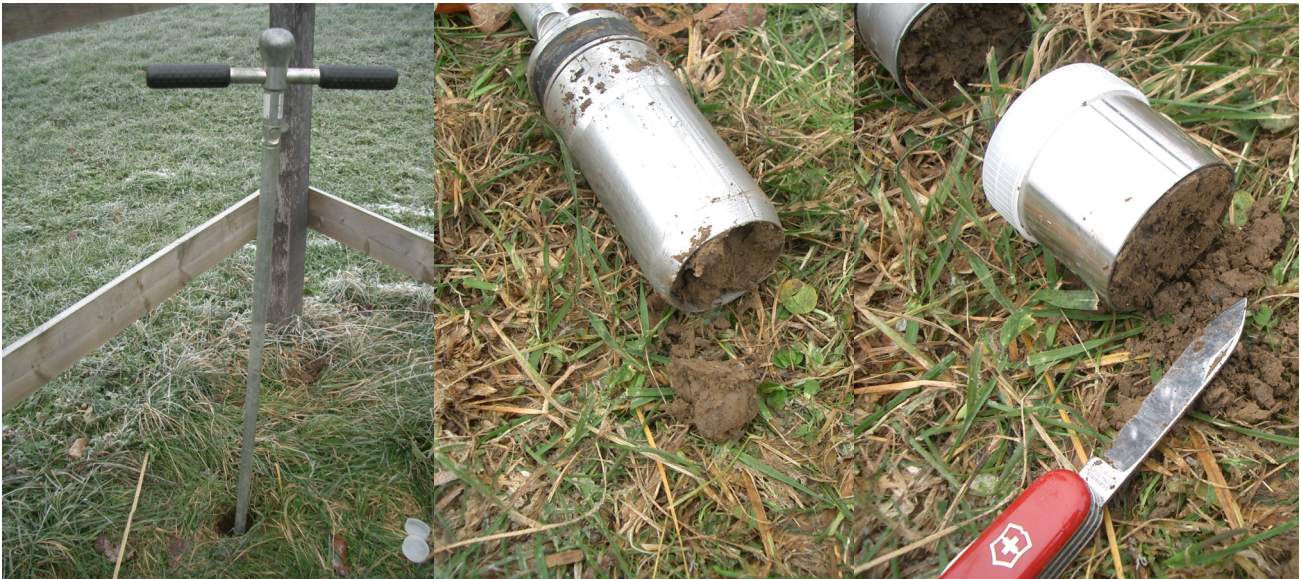
Figure 31: Soil sampling (from left to right): 1) hammering the closed ring holder into the soil, 2) removed ring holder with sample inside, 3) cutting off the excessive soil of the aluminium ring by knife.
