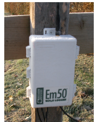
Fig. 24: Em50-Datalogger recording measurements of the 10HS-sensors.
