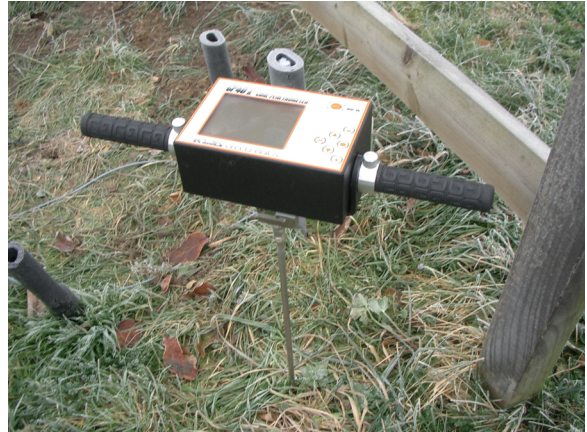
Figure 30: CP40II cone penetrometer inserted half-way in the soil.
