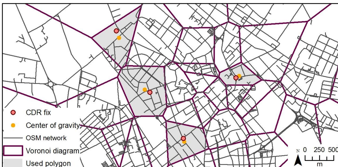
Figure 14: Center of gravity of the Voronoi cells used (subset of CDR data of user 4, 03.06.2013)
