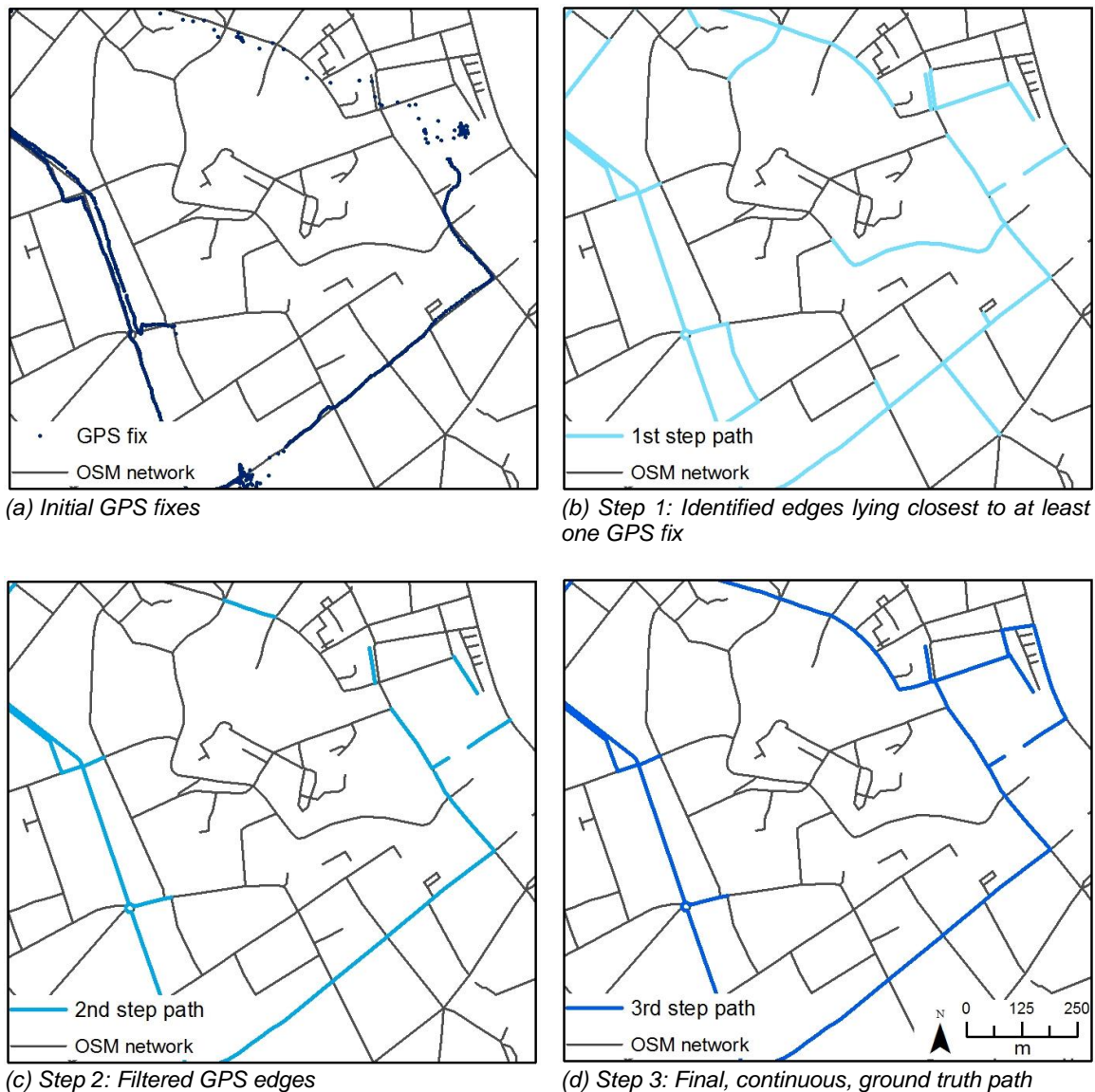
Figure 20: Visualization of initial GPS fixes and the three steps for deriving the continuous GPS path (subset of GPS data of user 4, 03.06.2013)
