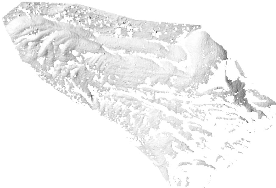
Figure 6.10: Result of the *Hillshade* function for the data set of the 5th of July 2013 with a DEM possessing a cell size of 1m.
