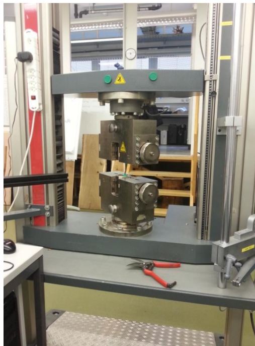
Fig. 3.6: The Zwick/Roell 100 universal testing machine at the ETH Hnggerberg. Photo: D. Kink, November 2013.
