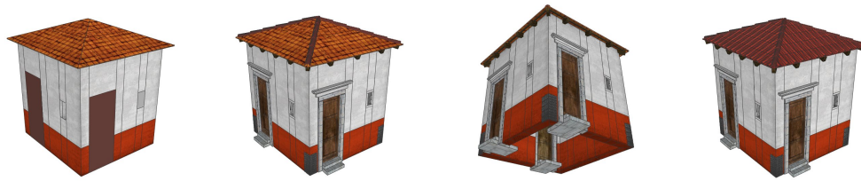
Figure 4.3: The Pompeii grammar rules with increasing complexity from left to right; LOD = 0 (quads only), LOD = 1 (doors and window elements), LOD = 2 (thick walls) and LOD = 3 (individual roof tiles), according to Maim et al. (2007)
