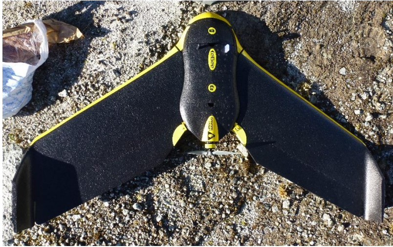
Fig. 18: The eBee drone by SenseFly used for the capturing of the aerial images.
